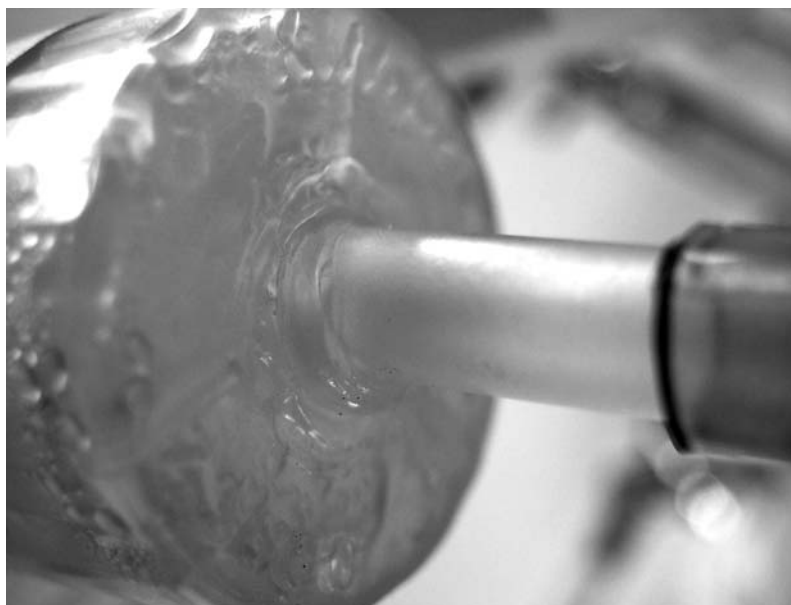
FIG. 3. Airstem weld using a commercial plastic welder. A plastic welder was used to partially melt the polypropylene tube and the top of the closure. While soft, pressure was applied to both ends of the tube in order bond it to the closure. Some distortion of the closure may occur, but this does not interfere with proper function.
