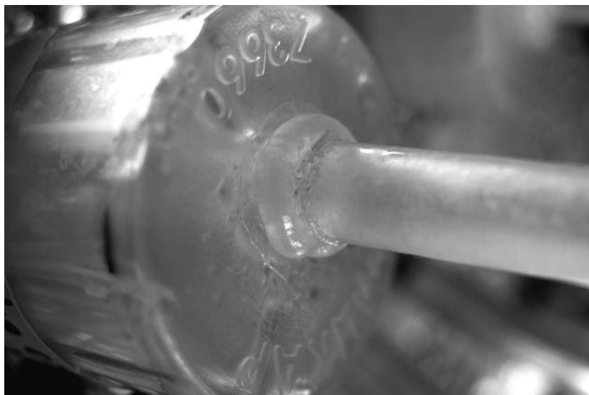
FIG. 4. Airstem weld using hot glue gun. A hot-melt glue gun was used to make this weld. A piece of polypropylene rod was used in place of the normal glue stick. This method is less expensive, and produces a neater weld. However, the weld usually is not as strong as one made with a plastic welder.
