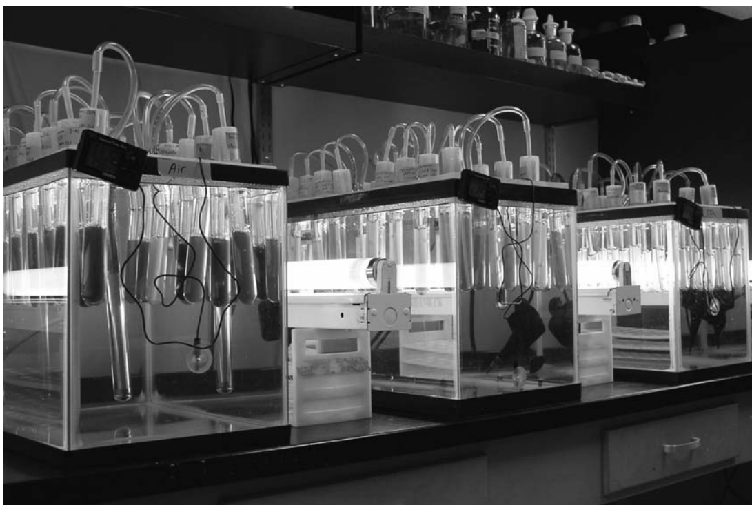
FIG. 2. Fully assembled culture tanks made from 10-gallon aquaria. Each tank supports 16 culture tubes. Lighting is provided by standard 24" cool-white fluorescent tubes. The black objects on the fronts are digital thermometers that record high and low temperatures and produce an audible alarm when the temperature exceeds a set range. As shown, each tank cost $100–$150 (U.S.) to construct.
