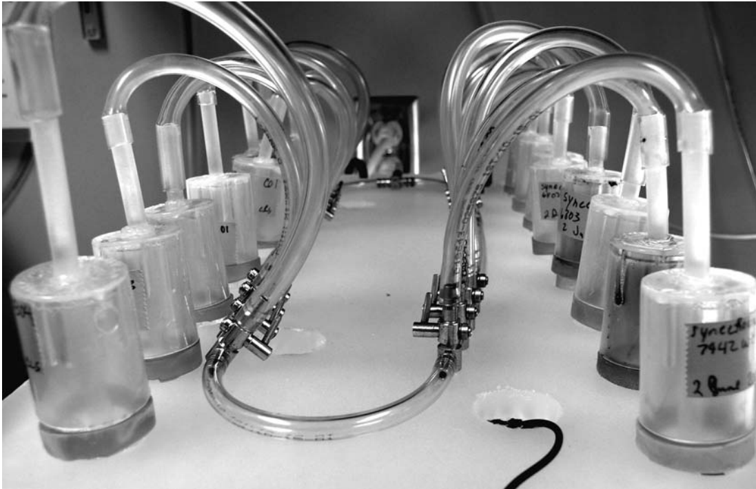
FIG. 5. Culture tubes attached to the gas manifold. Air or other gas is delivered via standard PVC aquarium tubing. A T-connector is used to split the delivery line into two sections, which are then joined at the front, forming a loop. Note the “rubber bands” below each closure, which prevent the culture tubes from falling through the cover. These were cut from \frac{3}{4} ” diameter surgical tubing. The black line in the foreground is a thermometer probe cable.
