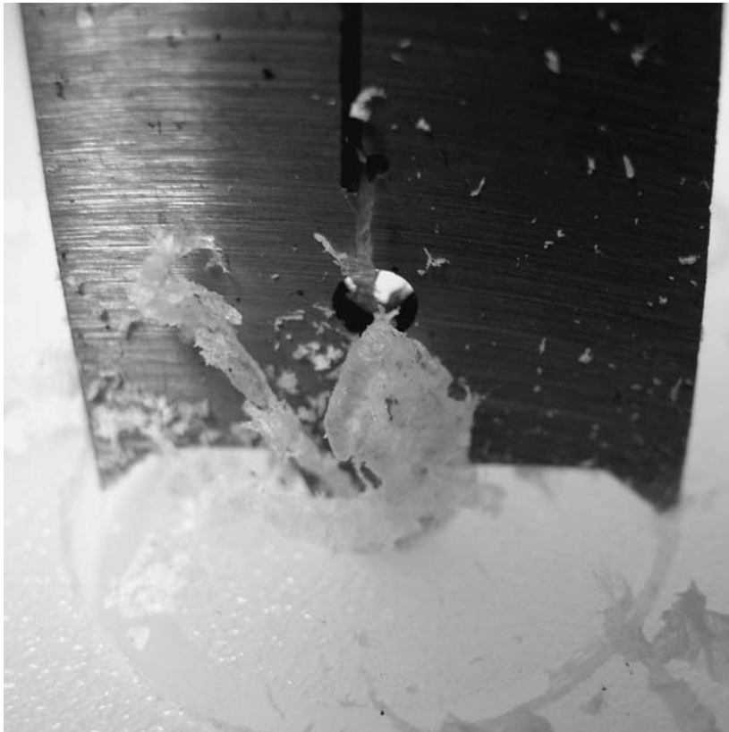
FIG. 6. Drilling a hole in the tank cover. A 1” spade was used to make holes in the polyethylene cover. In this case, the holes are just large enough for 25-mm-diameter culture tubes. Forstner bits or large twist bits would probably work as well, but hole saws generate too much heat, causing the plastic to melt instead of cutting through it.
